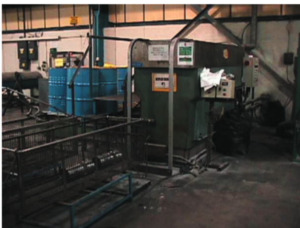
Figure 2 An industrial degreasing tank containing methylene chloride. This tank is fitted with a roller cover to reduce solvent vapour release into the work environment during operation. A number of workers have died when safe systems of work have not been observed during cleaning of such industrial degreasing units.
